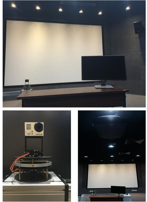
Fig. 2: Prototype system: photos of manipulator arms, digital camera, the slide rail, the 180-inch projection screen, 4k projector and TN LCD.
