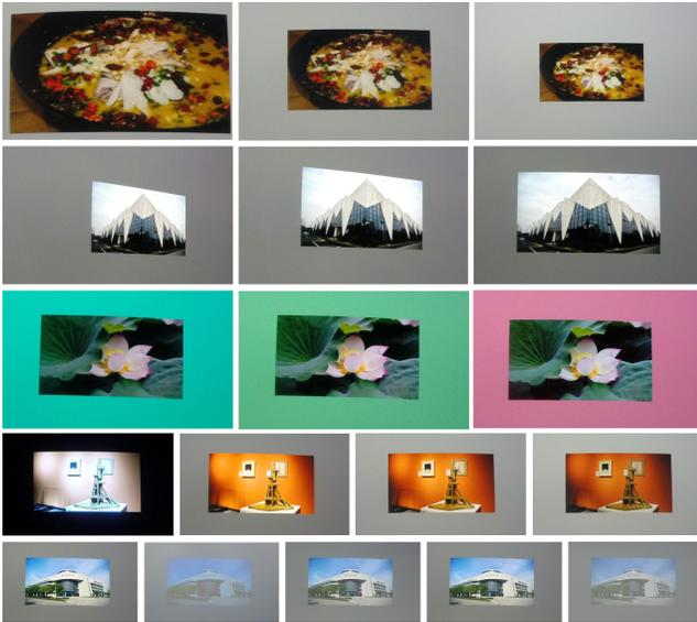
Fig. 4: The first row is of different distances. The second row is of different angles. The third is of different bias color temperature. The fourth is of different bias brightness. The fifth is of different room lighting.
